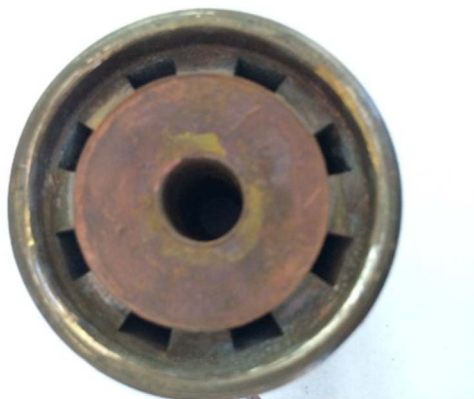
Fig. 3. The assembled evaporator with brass shell and copper powder sintered capillary wick.
